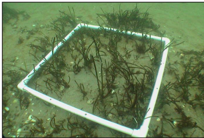
**Figure Intro-2.** A 0.10 meter<sup>2</sup> PVC quadrat used for eelgrass monitoring.
