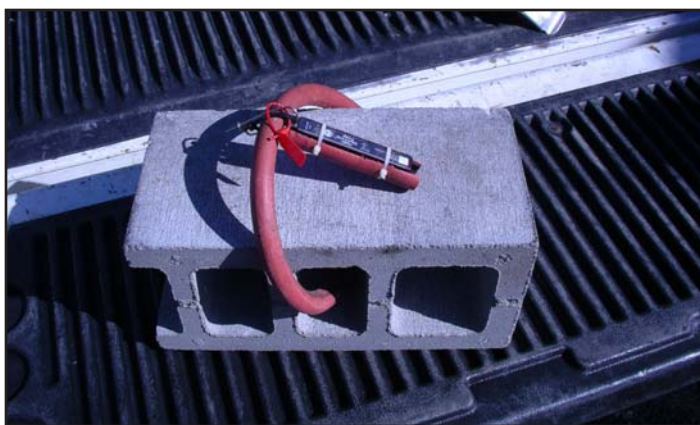
Figure Intro-1. A StowAway® temperature logger attached to a cement block, ready for deployment.
