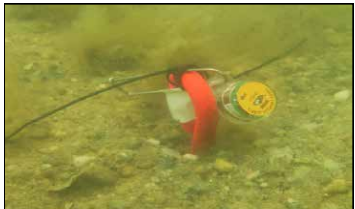
Figure Intro-2. A TidBit v2™ temperature logger attached to a screw anchor, deployed on-site.
