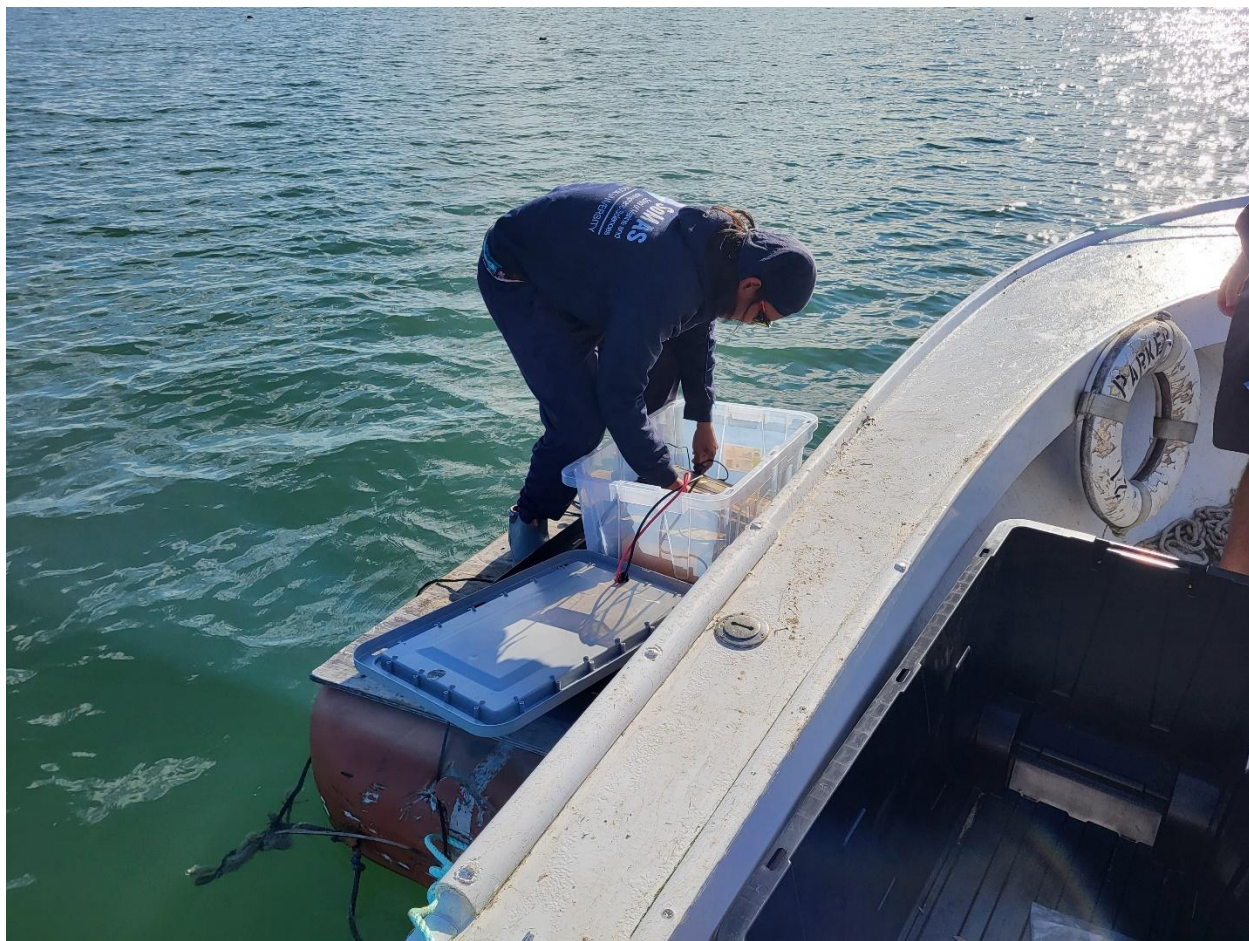
Supplemental Figures 8. Flexview Multibeam SONAR hardware set up on top of a life raft. Hardware includes 2 – 12v batteries, Toughbook laptop, inverter, positive and negative cables, external SSD, and SONAR power supply.
