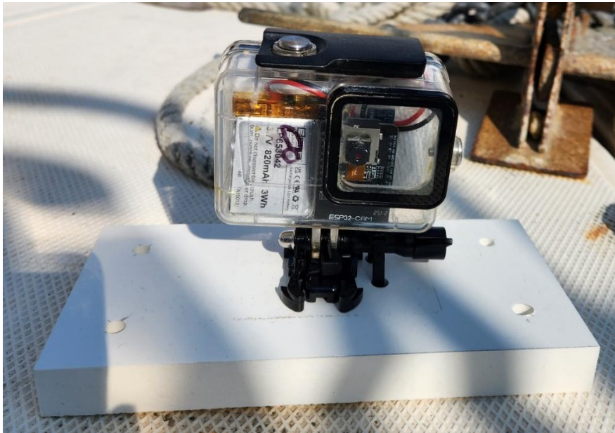
Figure 3. GoPro housing with KiloCam hardware, zip-tied to a 3/4" thick PVC sheet.
