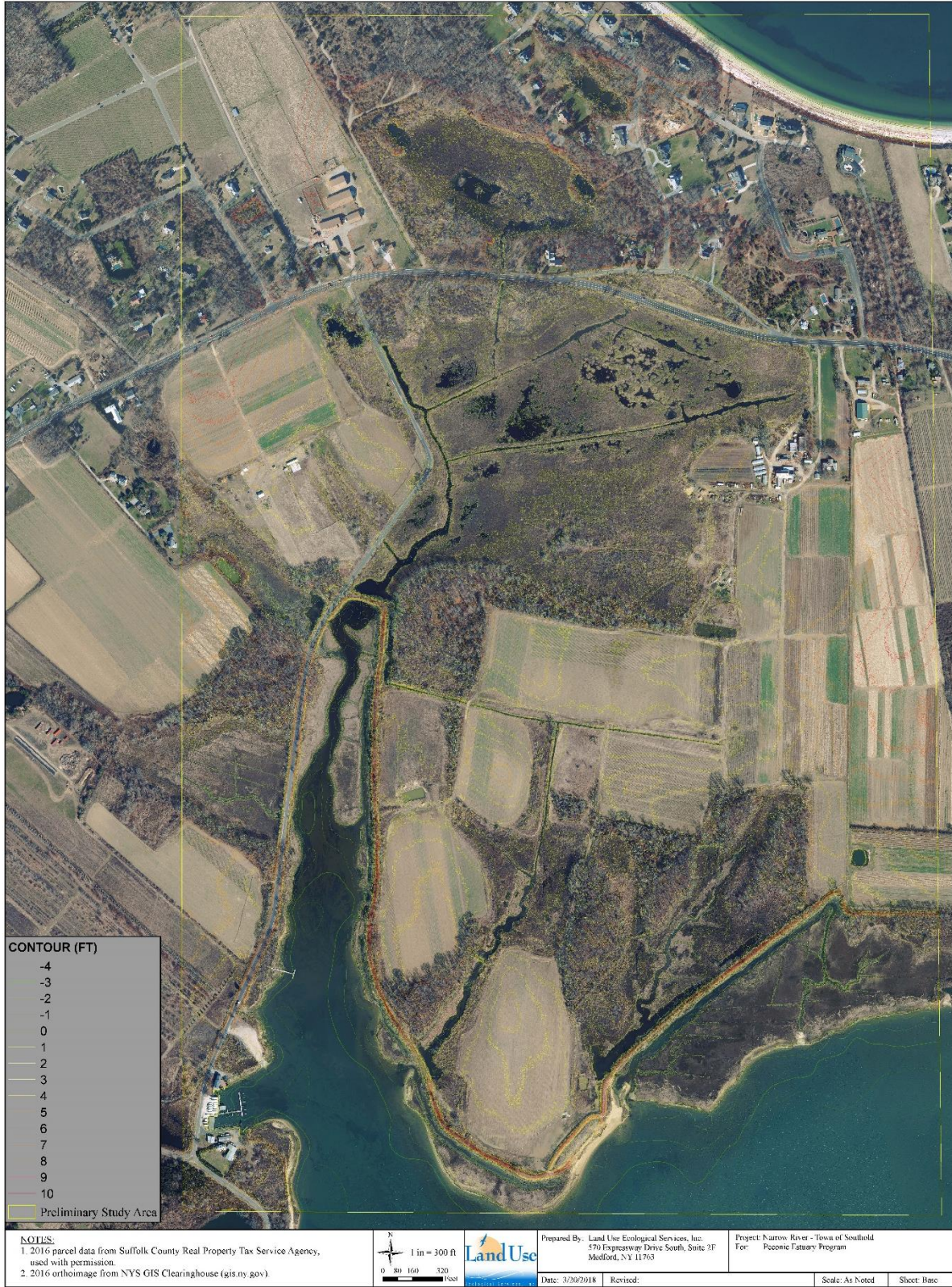
Figure 1: Narrow River topography utilizing 2016 USGS CoNED Topobathymetric Model (1887 - 2016): New England, obtained from the NOAA Data Access Viewer. Contour tool utilized in ArcMap on DEM.
