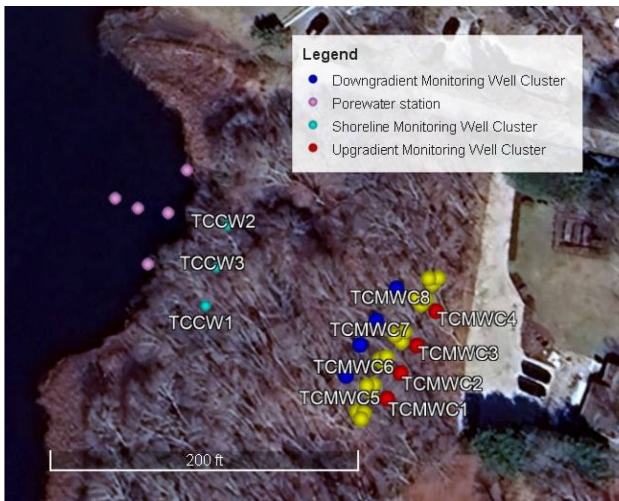
Figure 1: Tanbark Creek site schematic showing location of pilot PRB injection wells, upgradient and downgradient monitoring well clusters (TCMWC1-8). There are six injection clusters starting with TCINJ1 in the south and moving northeast to TCINJ6. The red and blue dots indicate 2 wells within 1 ft of each other screened at 20-25 ft and 10-15 ft below grade. Light blue dots represent shoreline cluster comprised of 3 wells screened at 5-15 ft, 15-25 ft, and 25-35 ft below grade. Light purple dots represent the 5 original long term monitoring offshore porewater stations.
