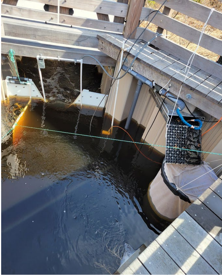
Figure 3. Viewing pool at Woodhull. Camera placed at fishway exit with reflective board on opposite side. Fyke Net collecting eels below eelpass.
