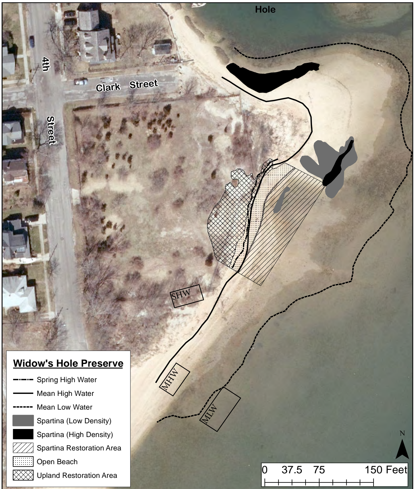
Figure 3. An outline of the proposed project components. The project proposes planting smooth cordgrass ( Spartina alterniflora ) from the mid-intertidal to high tide line. A section of open beach will be maintained between the cordgrass and American beachgrass (upland restoration area). An existing smooth cordgrass stand adjacent (northeast) to the project area that is being used as a biological benchmark and a small patch of smooth cordgrass growing in the proposed restoration area are highlighted.
