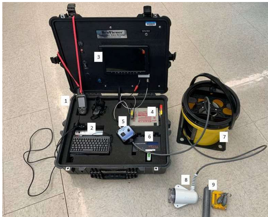
Figure 3. The underwater video camera system consists of several parts including video console (1-6) and camera (7-9): (1) Garmin differential GPS linked via cable and serial port to video overlay system (video water mark); (2) Proteus video overlay system with keyboard to input text (site name e.g.) on video files; (3) real-time video monitor; (4) external battery; (5) light controller and video capture settings; (6) digital video recorder with USB storage; (7) cable and management systems for tethered camera; (8) Seadrop camera; (9) down rigger weights. Not shown: camera stabilizing fin.
