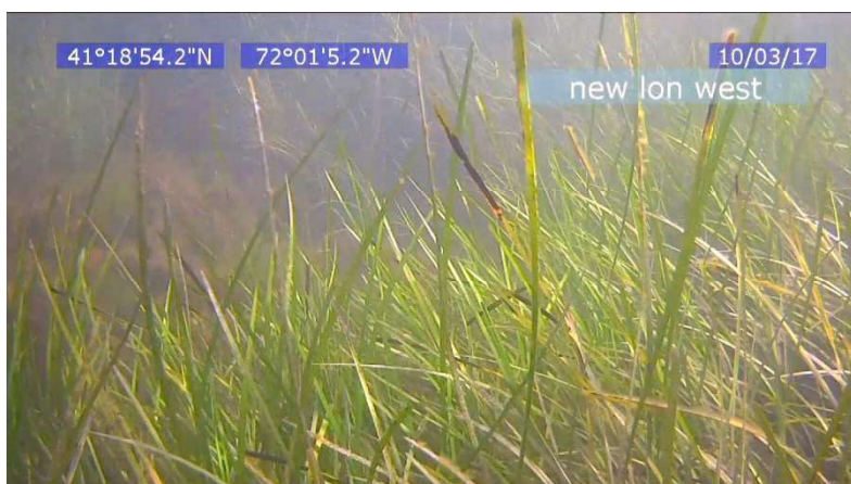
Figure 7. An example screen shot taken from an underwater video file. The python library tool py.tesseract interprets the lat long coordinates in upper left of the image and outputs them to a spreadsheet for use in ArcGIS.
