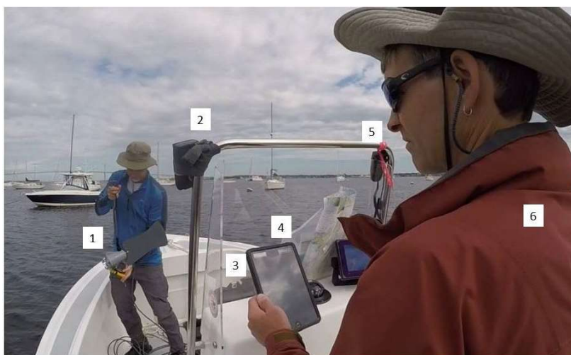
Figure 2. A photo of the eelgrass field survey set-up including the underwater video camera (1) and console including real-time video feed (3), the sub-meter GPS (2) linked to tablet (4). GPS used for video water mark, and intrepid boat captain (6).
