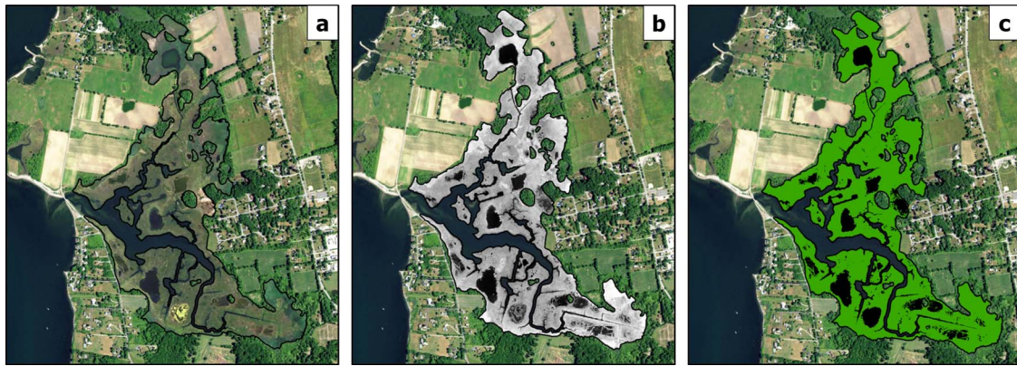
Figure 2. Image classification workflow to assess the unvegetated:vegetation ratio developed by Ganju et al. (2017), demonstrated for Sapowet Marsh site in 2016: (a) National Agriculture Imagery Program, (b) normalized difference vegetation index, (c) supervised pixel classification to unvegetated (black) or vegetated (green) marsh surface and manual reclassification of shadows and floating algae.
