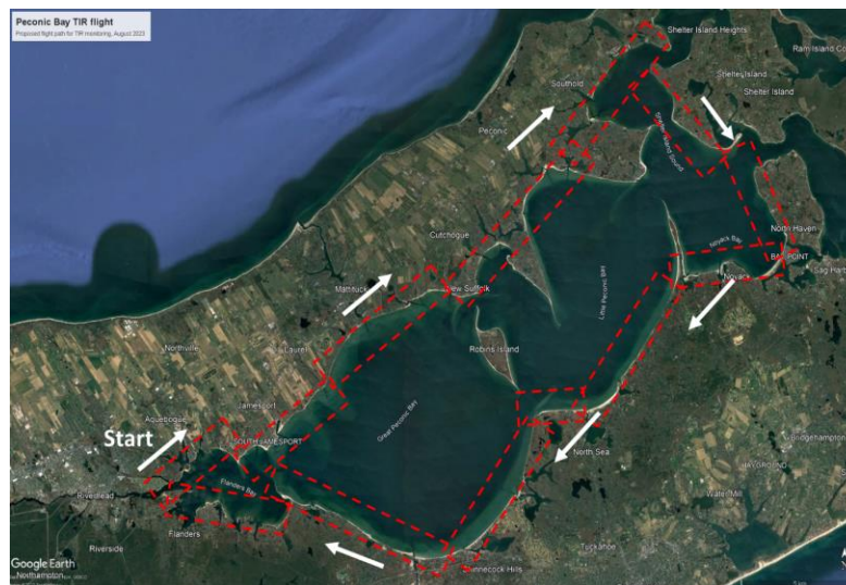
Figure 3. Map of Peconic Bay with proposed TIR overflight track for August 2023. The initial survey will be at ~2000 m altitude before targeting the six regions of interest from the USGS model output (~1000 m altitude). The width of the red-dashed rectangle is approximately representative of the image swath at 2000 m.
