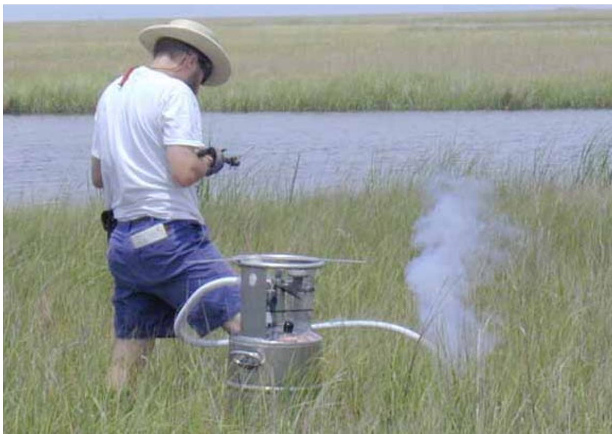
Figure 5.34. Taking a cryo-core. Note white cloud from the \text{LN}_2 escaping the bullet (Fire Island NS, New York, NY USA).
