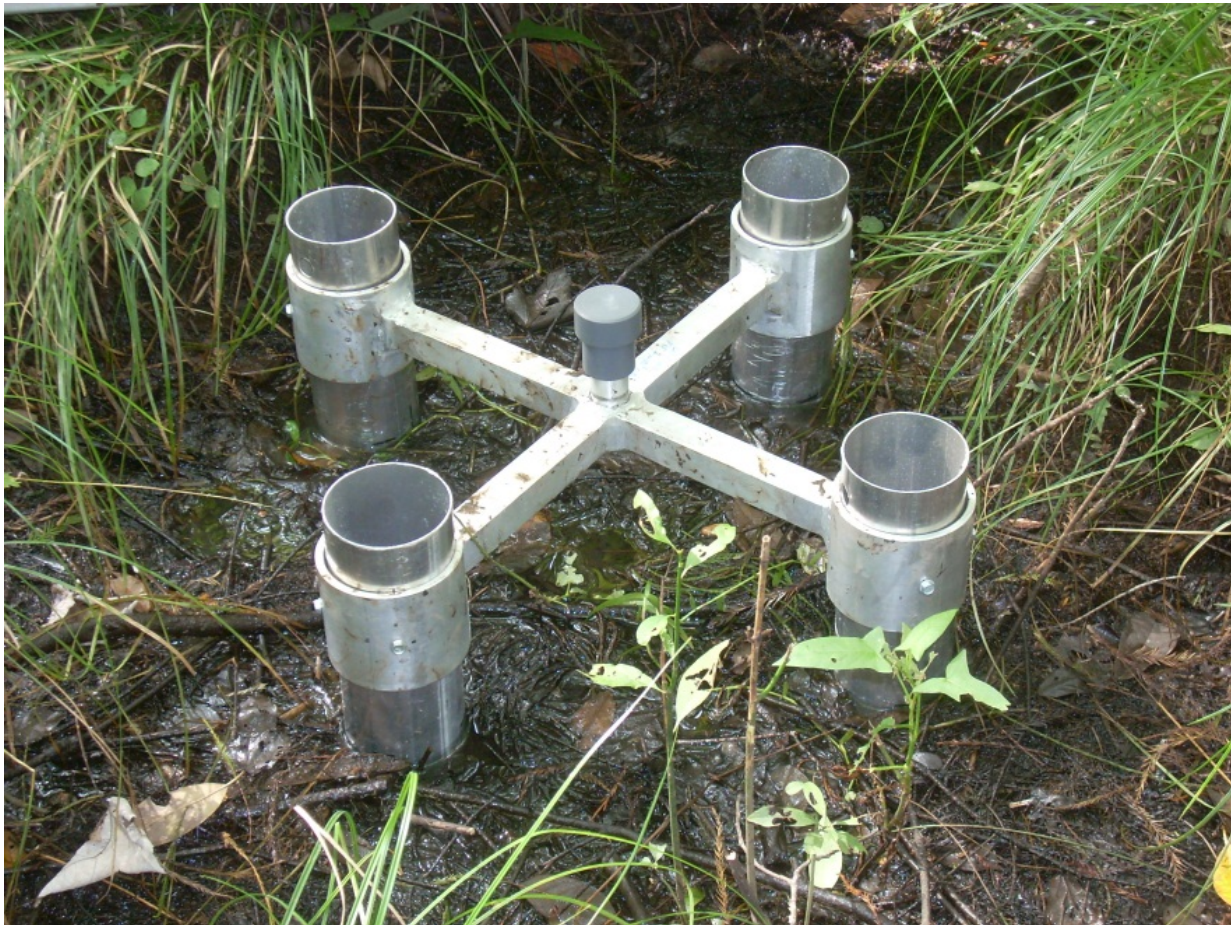
Figure 3.35. Completed installation of a shallow SET platform. Note that the legs are now attached to the framework with screws.
